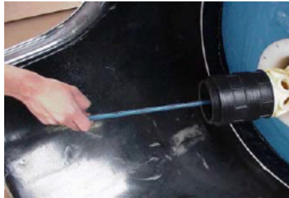
Step 2: Parts shown in Step 1 are assembled (outside of tank) and inserted in tank using extension I-WR03-LA.
